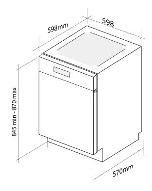
Note: For built-in installation, please remove the lid of the appliances. Refer to the installation manual
